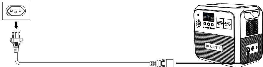
AC180 supports Turbo/Standard/Silent charging modes. It's set to standard charging by default, while the Turbo and silent modes can be enabled in BLUETTI app. BLUETTI's AC charging mode guide is as follows:
