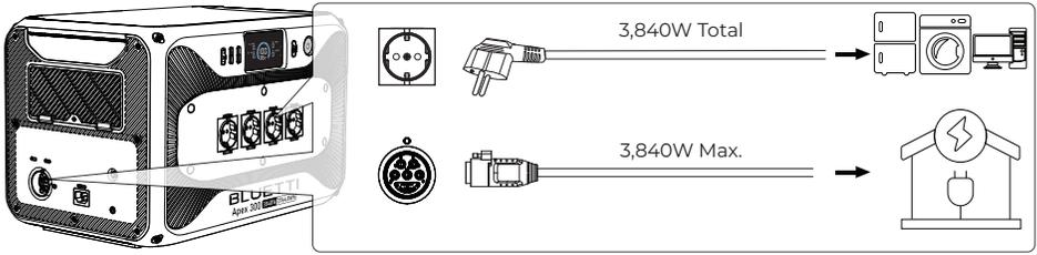
**Note:** When servicing the devices connected to the unit, remember to unplug them from the outlets. Even if the AC output is turned off, physically unplugging the devices is necessary for complete disconnection.
