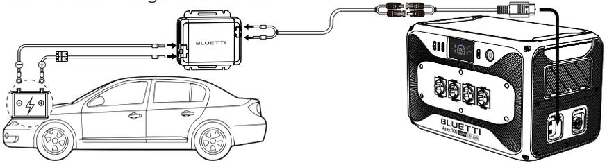
**Note:** Make sure your car has power and the engine is running while charging to prevent over-discharging the car battery.
