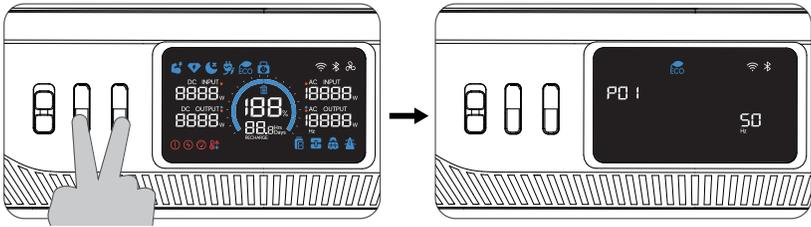
**Exit the Mode:** Press and hold both the AC power and ECO mode buttons again. If left idle for 1 minute, the Apex 300 automatically exits without saving any changes.
