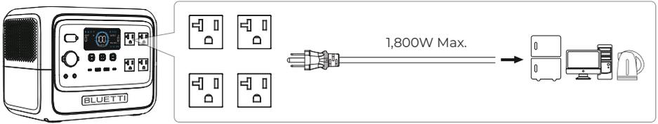
**Note:** When servicing the devices connected to the unit, remember to unplug them from the outlets. Even if the AC output is turned off, physically unplugging the devices is necessary for complete disconnection.
