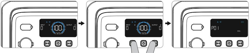
**Exit the Mode:** Press and hold both the AC and DC power buttons again.
