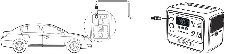
**Note:** Make sure your car has power and the engine is running while charging to prevent over-discharging the car battery.
