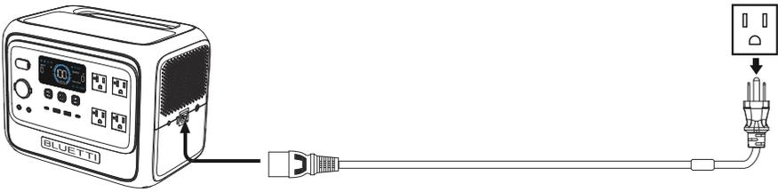
**Note:** Do not plug the unit's AC charging cable into its own AC outlets, as this could damage the connected device.
