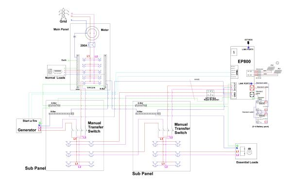
Note: The EP800 electrical diagram has no CT on the grid side.
